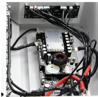
Built-in intelligent BMS system
